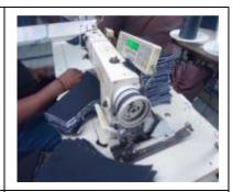
NC: pulley guard not installed on machine
